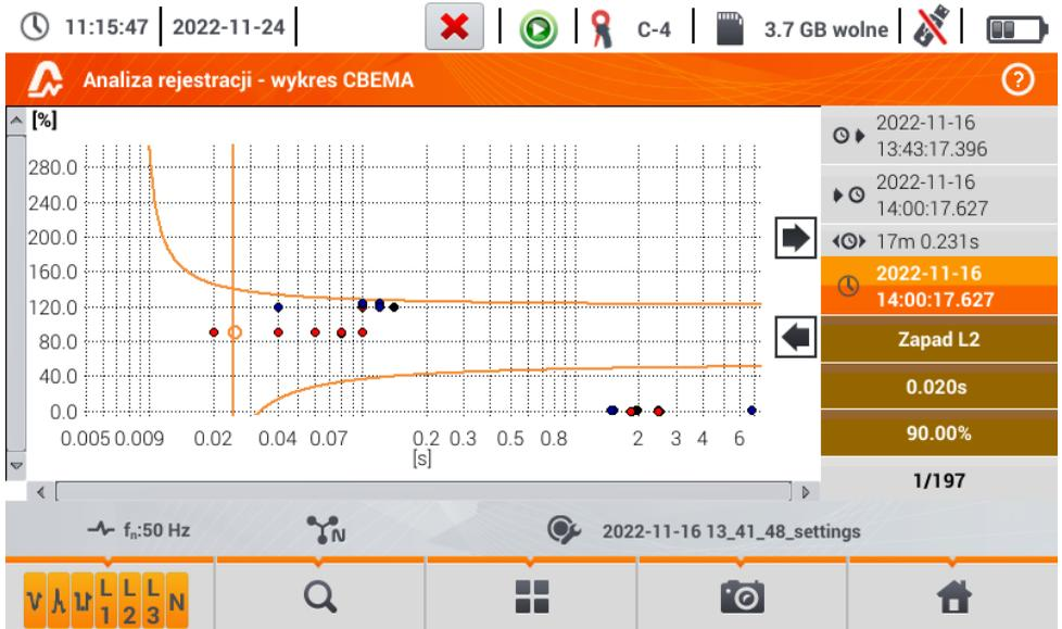
Fig. 5.27. Recording analysis – CBEMA graph
